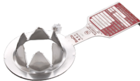
After bursting of LF Rupture Disc
